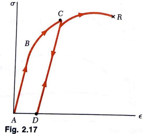
A body that is plastically deformed and then released, undeforms or springs back toward its original shape. Consider bending of a metal plate between a male and female die or through offset rollers:
