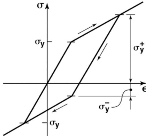
Figure 2-36 Bauschinger Effect for a Linear Strain-Hardening Curve
