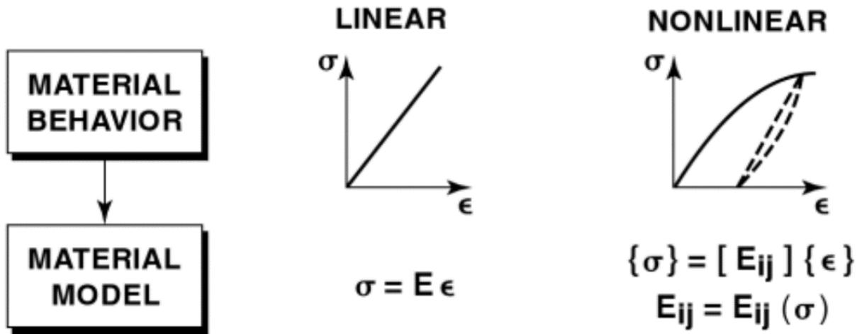
General nonlinear behavior of engineering materials can be explained by evaluating properties like ductility, yielding, energy absorption, unloading behavior, elevated temperature behavior, bimodular behavior, anisotropy
