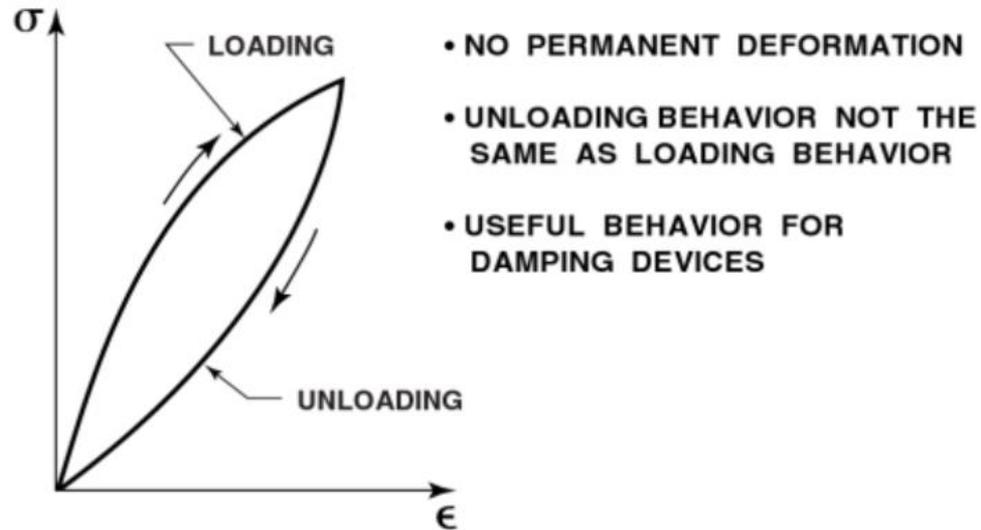
This behavior is different than elastic behavior because the loading and unloading curves are different, plastic.
