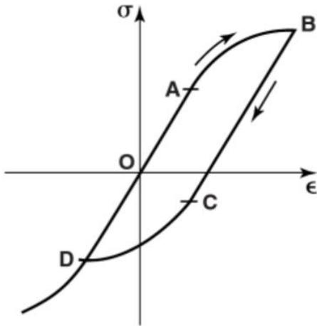
Figure 2-35 Bauschinger Effect for a General Linear-Nonlinear Curve
