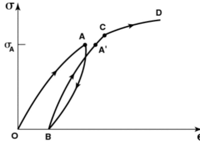
The loading history affects both material microstructure and the resultant stress-strain curve
