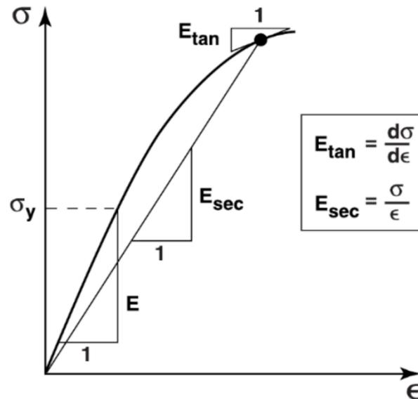
The secant modulus is just a representation that if we know the nonlinear stress level and the modulus, then we can calculate the strain
