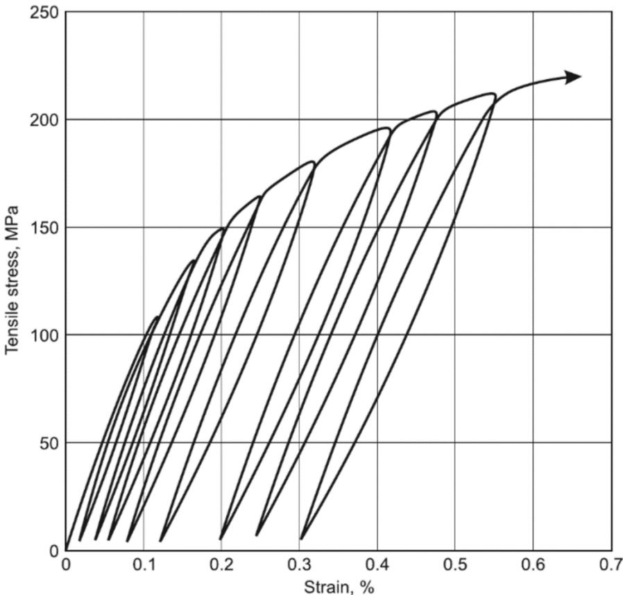
**CI.052 Flake graphite, gray iron casting, tensile stress-strain curves with cyclic loading to increasing stress levels**
