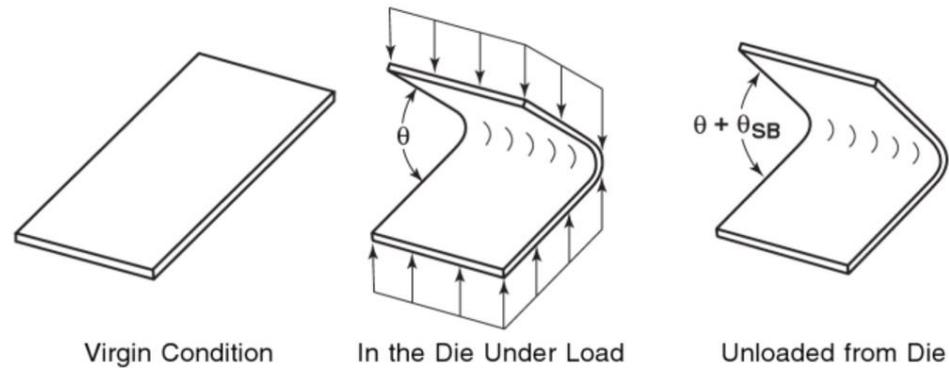
The reason for the springback is the elastic strain that is recovered during unloading
