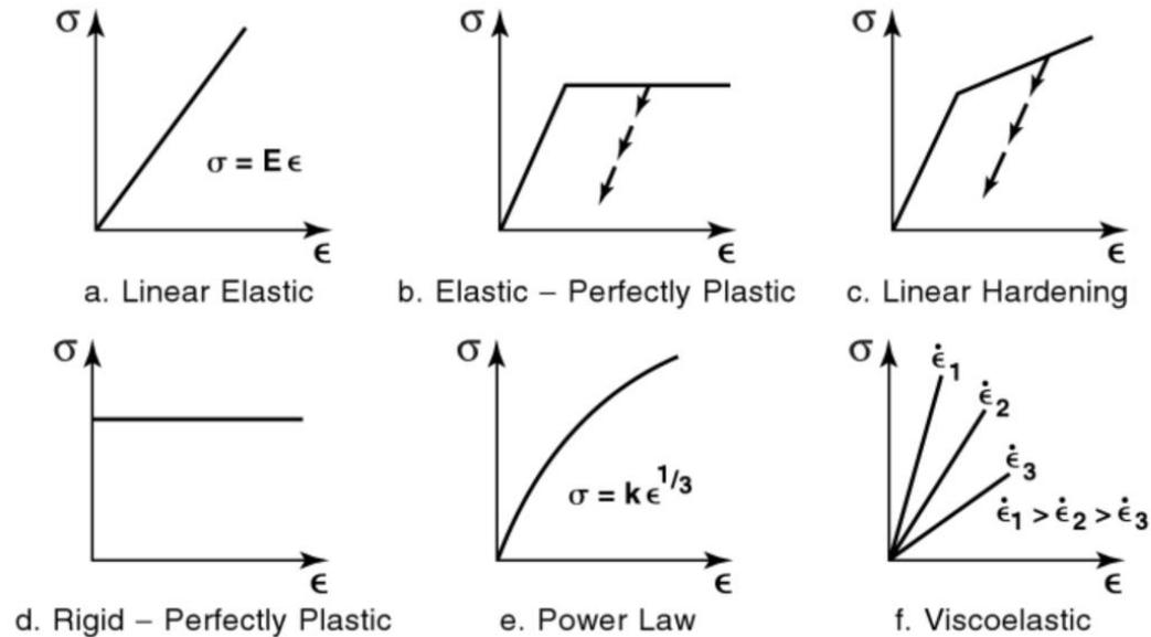
The simplest is the linear elastic approach in which only two material parameters  $E$  and  $\nu$  are needed for the model
