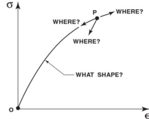
The stress-strain curve shape is generally a function of the material, temperature, loading rate, and many other factors that we will consider
