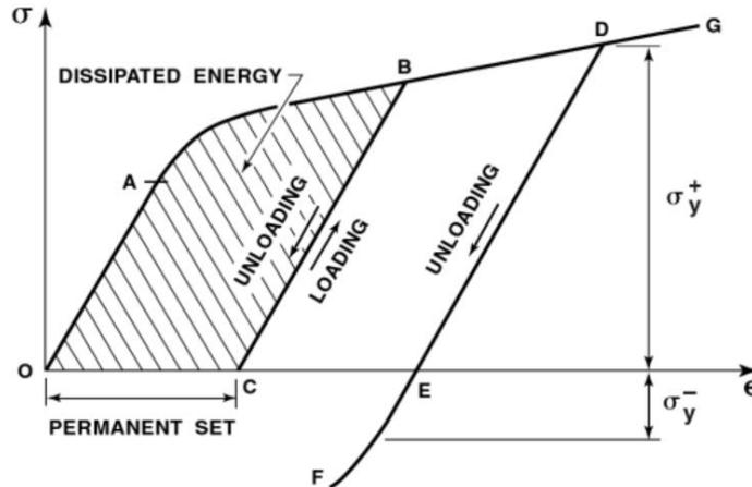
The loading and unloading cycle produces some strain hardening, permanent deformation and an associated springback effect
