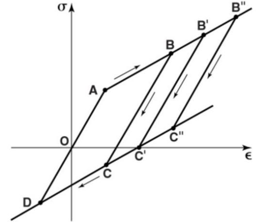
Figure 2-37 Bauschinger Effect for a Linear Strain-Hardening Curve with Multiple Load-Unload Cycles
