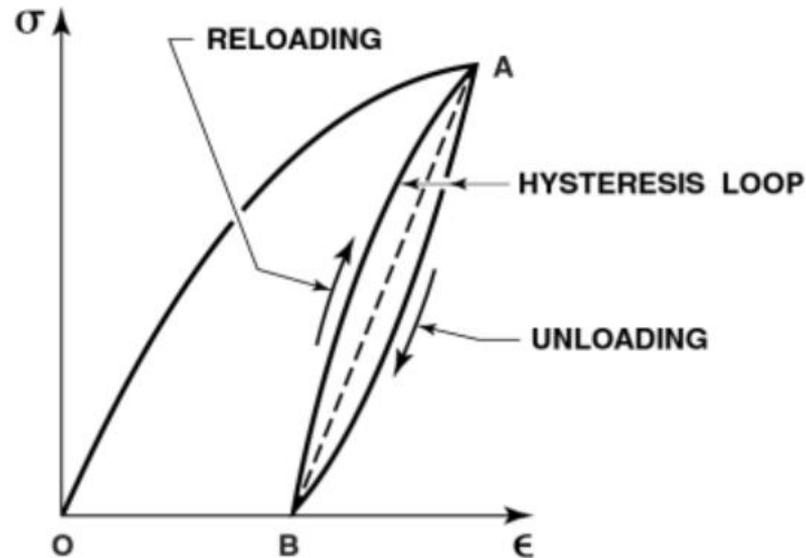
Typically there is a difference between the unloading curve and the reloading curve, a hysteresis loop is seen that indicates that energy is dissipated.
