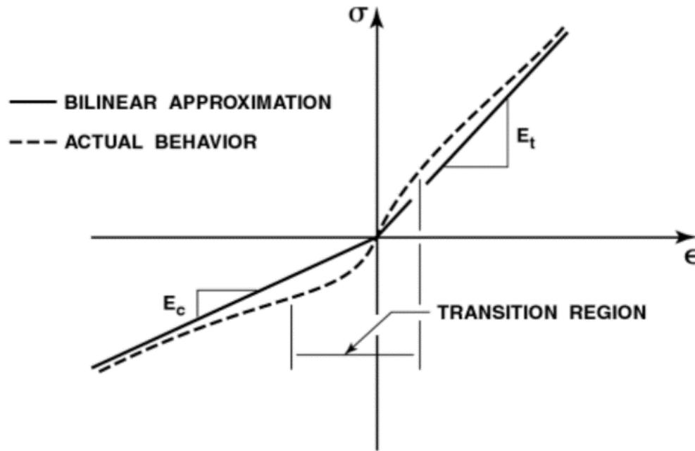
Unloading of materials after loading and the way they behave during unloading affects their deformation behavior upon further loading
